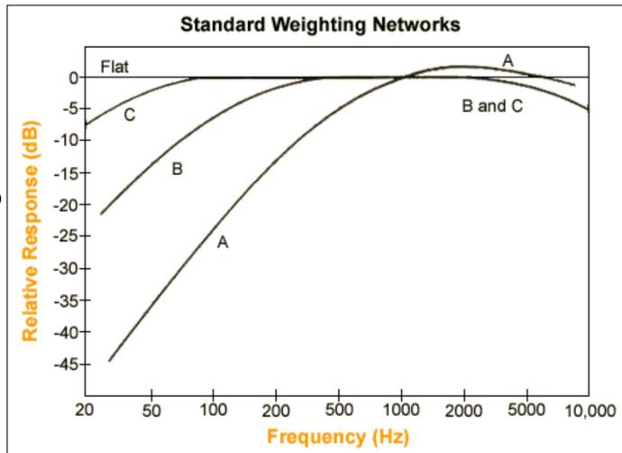
By using these weighting networks, the measuring instrument is able to respond to some frequencies more than others.
