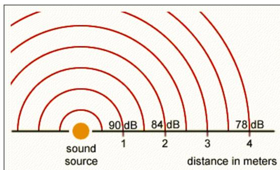
**If a point source in a free field produces a sound pressure level of 90 dB at a distance of 1 meter, the sound pressure level at 2 meters is 84 dB, at 4 meters is 78 dB, and so forth.**
