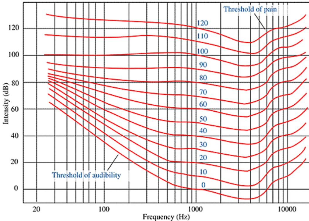
Look at the curve for 40 dBA. Find 30 Hz. It is the line immediately to the right of 20 Hz.
